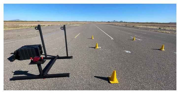
The FMVSS 108 test requires a lane width of 10ft – 12ft. All lanes setup at AMTC for this test are 12ft wide. To verify that our lanes are within spec, we laid them out using survey equipment which has accuracy levels to centimeters. Physical markers with associated GPS coordinates are used to layout the lane for simplifying test setup and data analysis.
